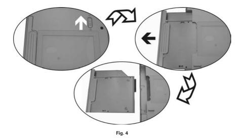
The module in the multifunction slot can be replaced with either a CD ROM module, a DVD module, a second battery or a SATA hard disk.
